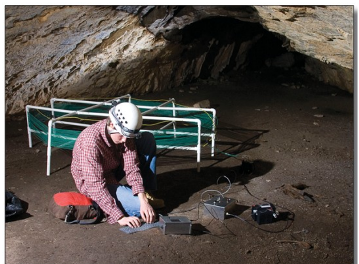
Figure 3. Photo of the underground radio set up in Black Cave, Eddy County, New Mexico. This was the configuration used for communication as well as obtaining signal strength measurements.
