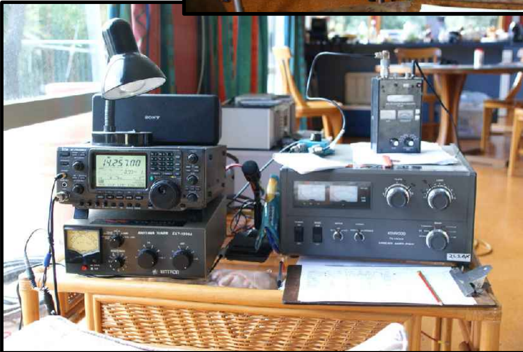
Operating Station No. 2 IC-746 PRO + Kenwood TL-922 Linear
