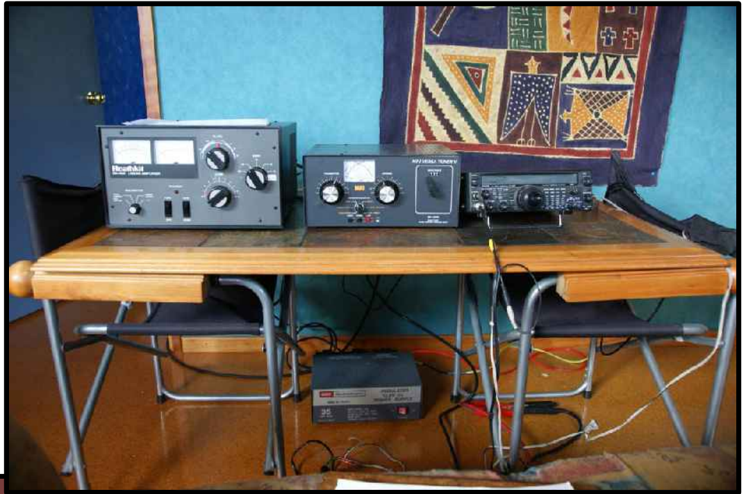
Operating Station No. 1 FT-847 + SB-1000 Linear
