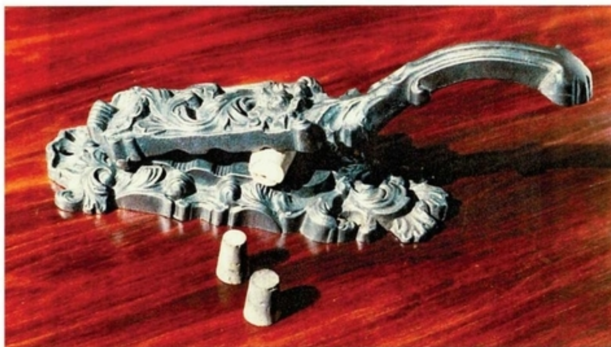
This ornate cast-iron cork press was for softening corks before they were used to seal prescription bottles. A. KENRICK & SONS of London was the foundry which made this pharmaceutical cork-press.
