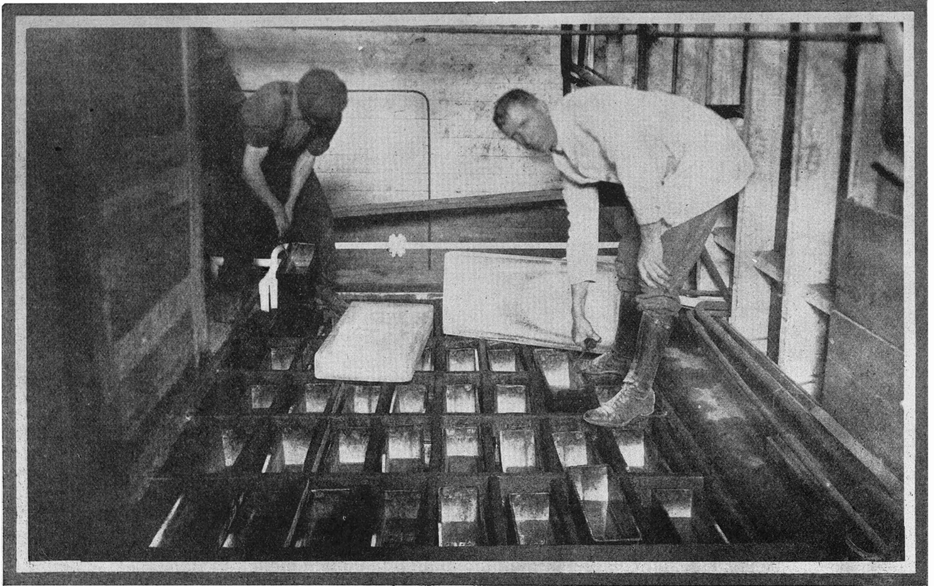
Lowe's Limited specialise in Ice making—view showing part of Ice making Machine capable of turning out 2\frac{1}{4} tons per day.
