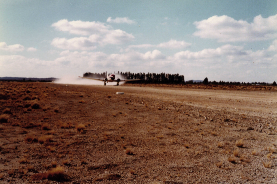
James Aviation Ltd, - Douglas Dakota (DC3) topdressing aircraft taking off with 5 tons of farm fertilizer. Pilot - Les Marshal. Rangitaiki airstrip. : October 1973.
