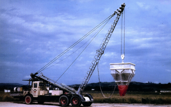
James Aviation Ltd, - Douglas Dakota (DC3) aircraft loading device mounted on a Thorneycroft 6x6 truck. Hopper capacity 5 tons - (DC3 aircraft load). : 1972.
