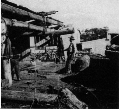
Odlin Timber & Hardware Ltd , sawmill - Pohokura. Napier Taupo Road, 'Skiddy' Barry Gore about to roll log into mill - breaking down carriage. Photo : December 1959.
