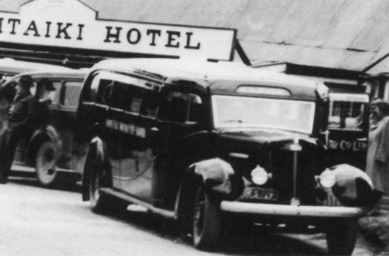
Hawke's Bay Motor Co, - services cars Rangitaiki Hotel about 1946 - 47. This type of service car often referred to as side loaders - multiple doors along left side. A "WHITE" chassis - body built in Napier by Nuttall coach builders.
