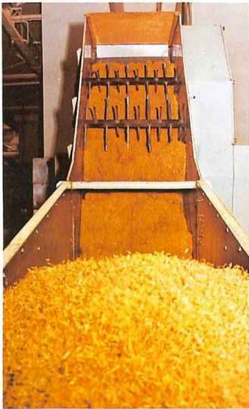
Blended cigarette tobacco is cut to the finest tolerances prior to transfer to cigarette making machines.
