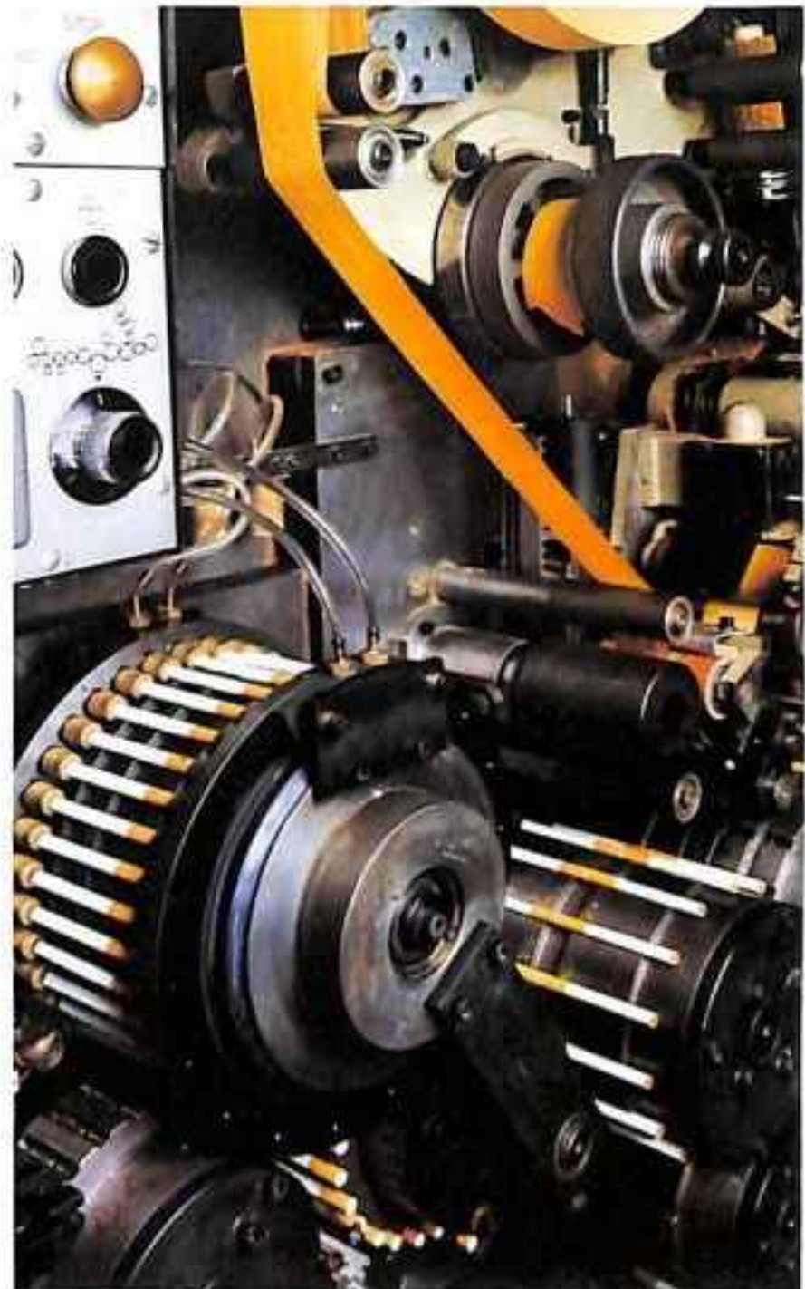
Highly sophisticated machines attach filter plugs and cork tipping at speeds of over 4,000 cigarettes a minute.
