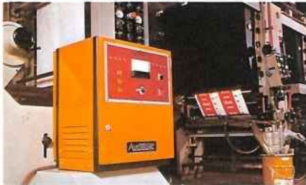
10 hp variable speed controller fitted to a printing press.
