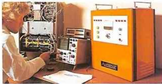
Final circuitry check of an AC motor speed controller.
