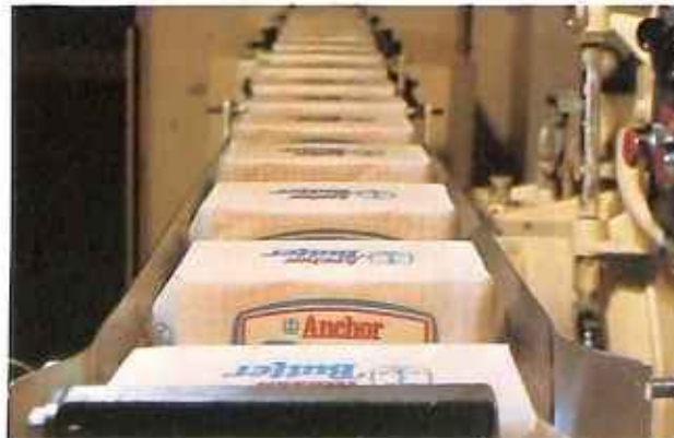
High speed butter packing equipment at Auckland Co-operative Farm Products Limited patting plant fitted with a motor controller.
