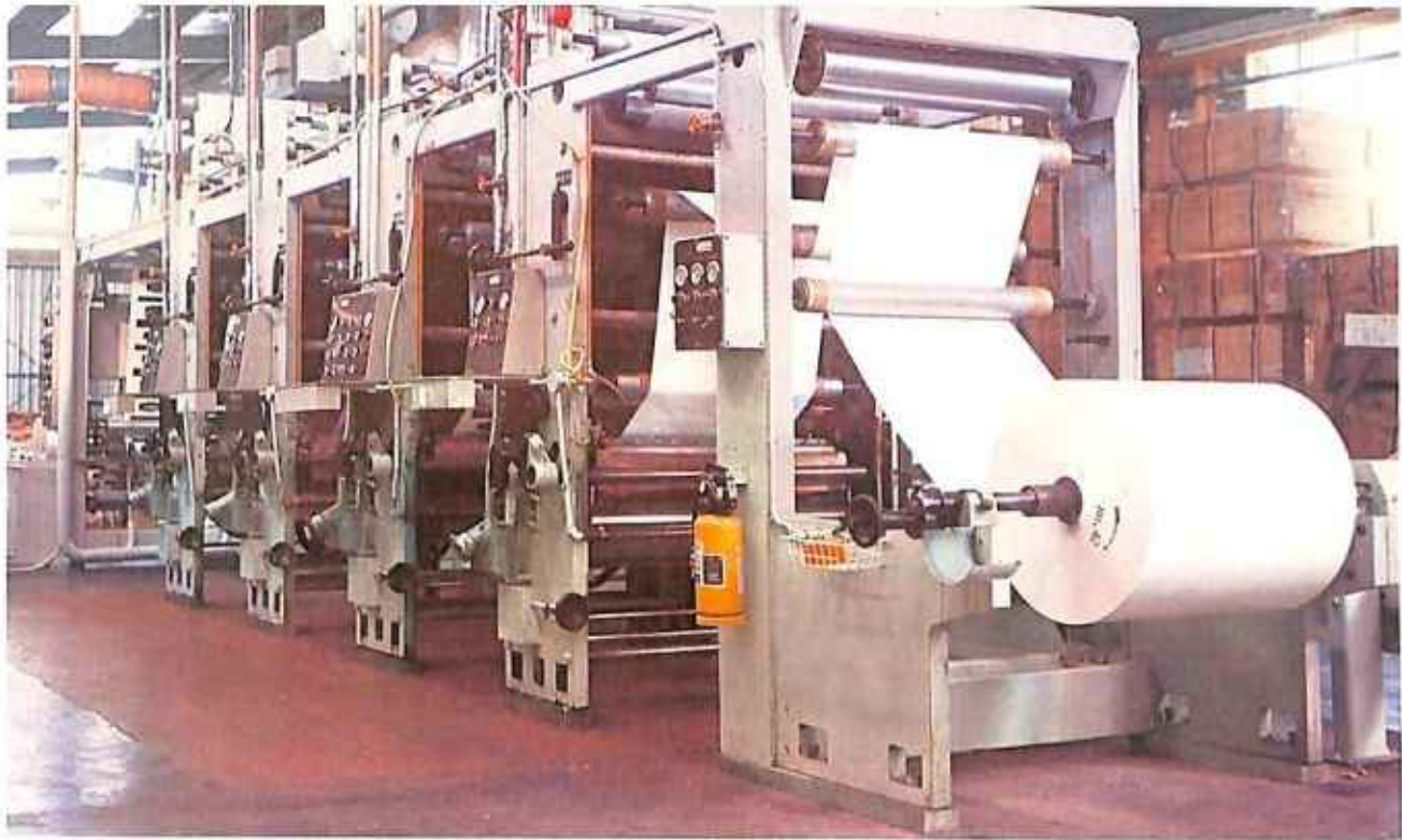
Printing Hall showing 4 station gravure press.
