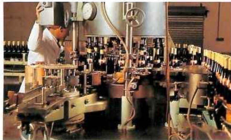
Automatic labelling at speeds up to 10,000 bottles an hour.
