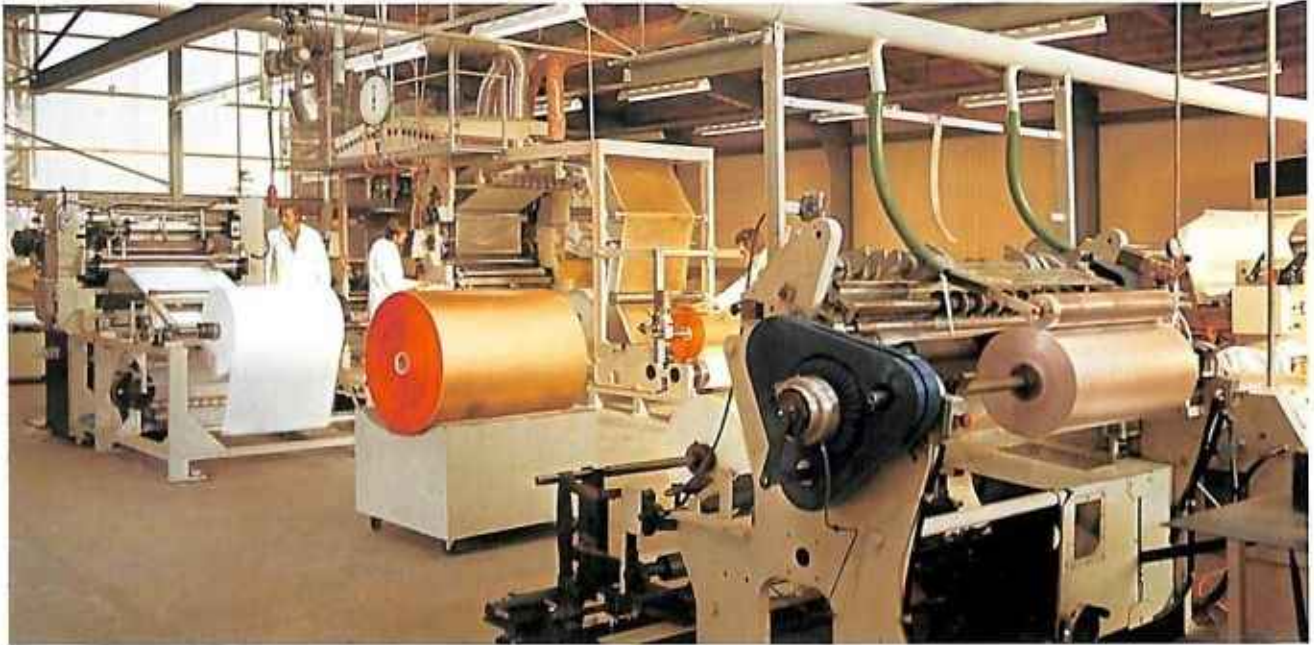
High speed lacquering and laminating plant.
