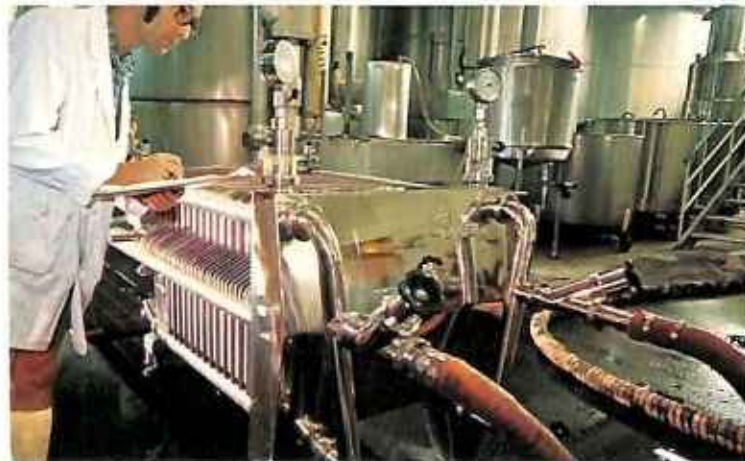
For perfect clarity wines are given a final polish through micro filters.
