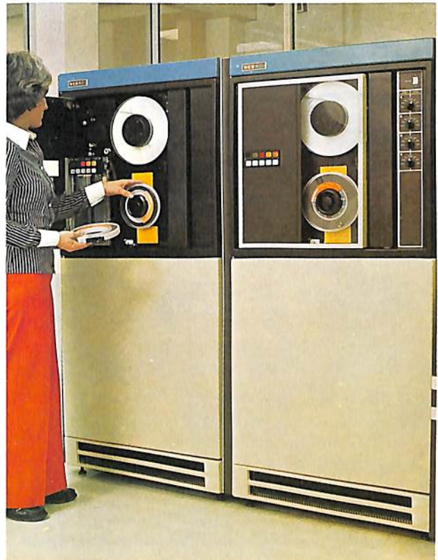
Above – High speed tape handling units. Below – Keying data for processing.
