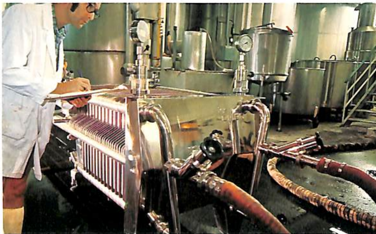
For perfect clarity wines are given a final polish through micro filters.
