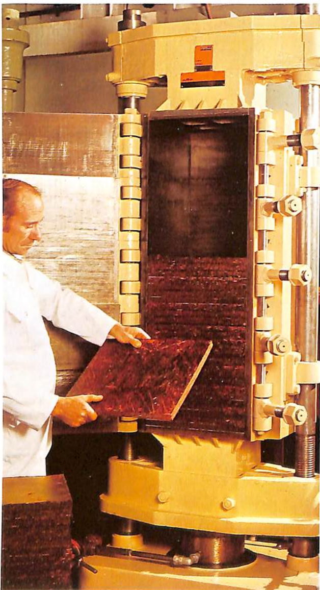
Removing pressed cakes of Erinmore Flake pipe tobacco prior to slicing and packing.
