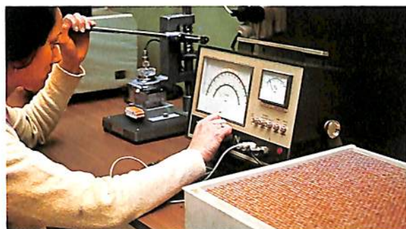
Routine moisture testing by electronic equipment is essential in maintaining the superior smoking qualities of fine tobaccos.
