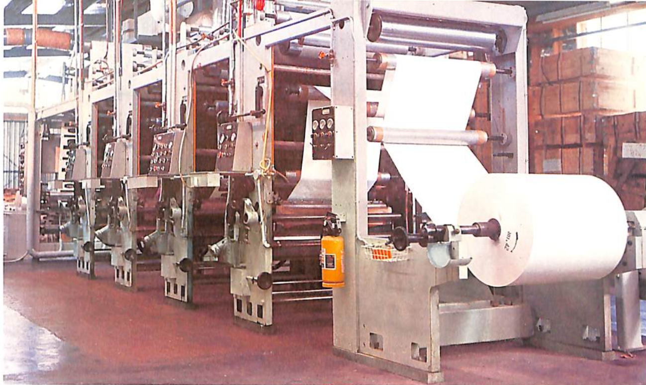
Printing Hall showing 4 station gravure press.
