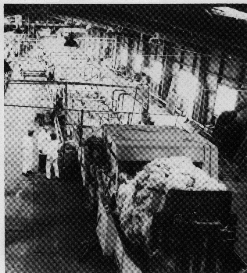
The main scouring train at Tomoana showing the fork lift [at bottom] loading wool into the hopper.
