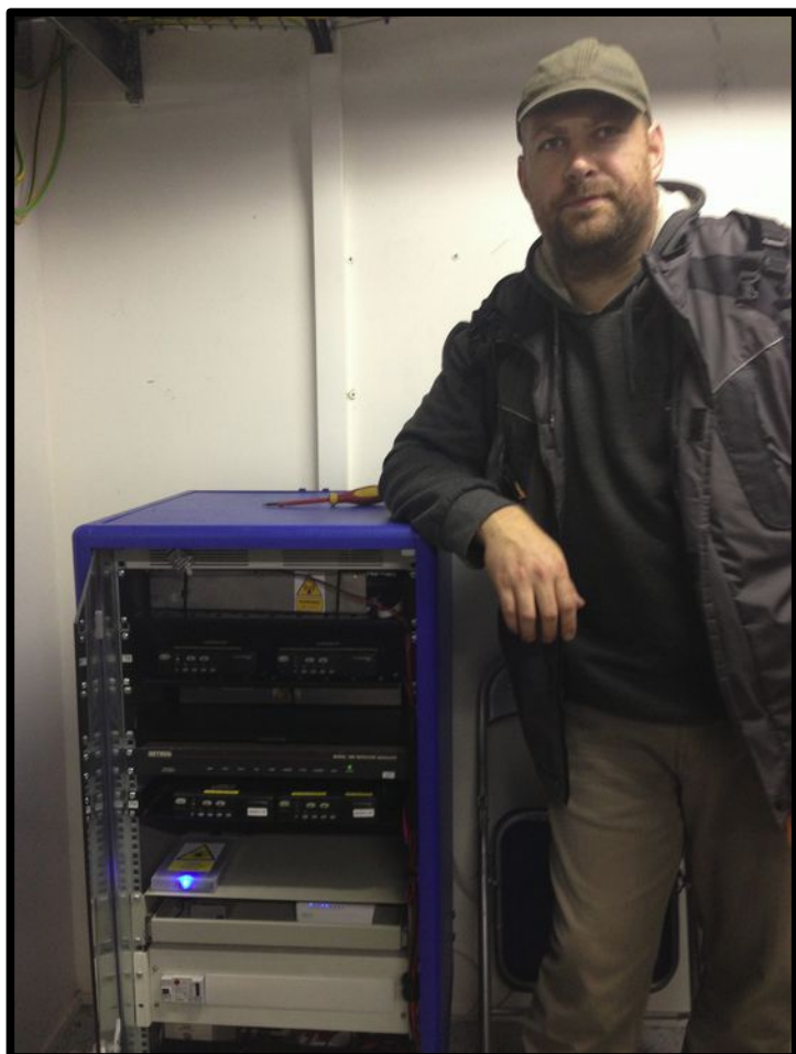
Tom OK1JRA with a digital/analog combined repeater he built
