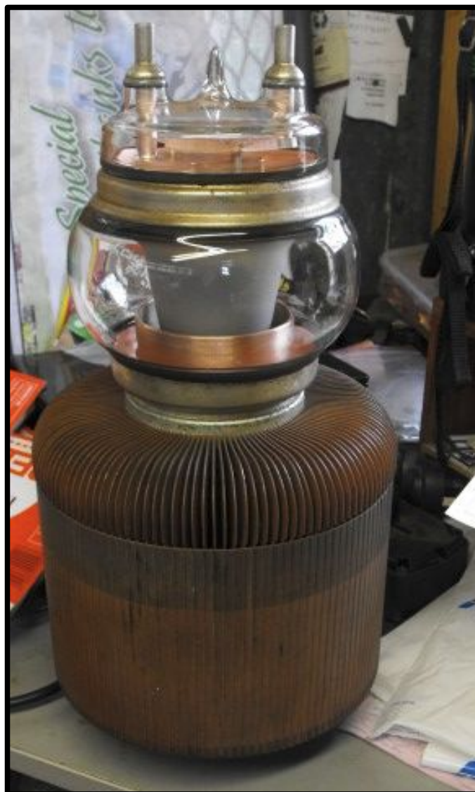
Valve final, believed to be from Opapa, HB broadcast radio station. Much of what you can see are copper cooling fins
