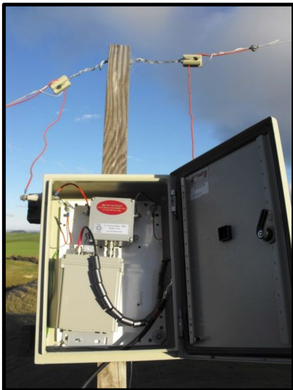
outside box showing the mocked up Ant. feed point 4:1 balun/Auto Tuning Unit/1:1 choke balun arrangement
