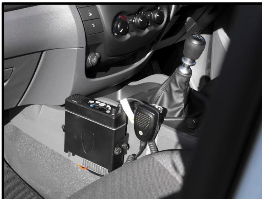
Commercial Mobile R/T installed in a Ford Ranger
