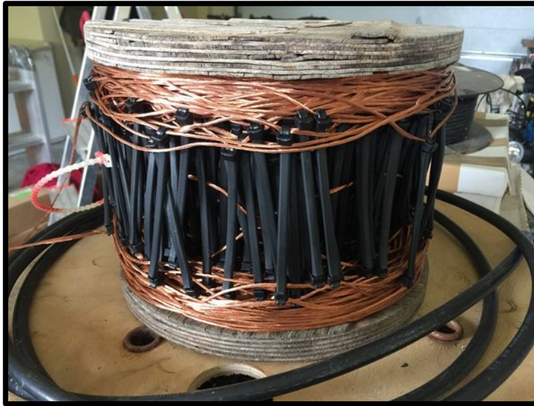
Figure 7: 600 Ohm line, stranded copper wire using cable ties & heat shrink method
