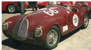
1940 Autoavia 815. Italian entry. The second Ferrari designed vehicle to be built. 8 cylinder 1.5 litre.
