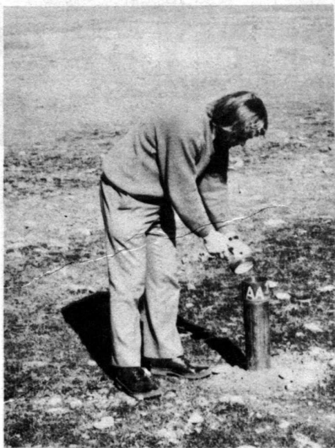
Checking the level of water passing under the ground.
