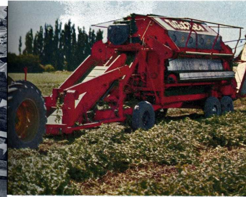
Pea Harvester in action delivering shelled peas into bins on the move, at a rate of 8 tons a day per machine.
