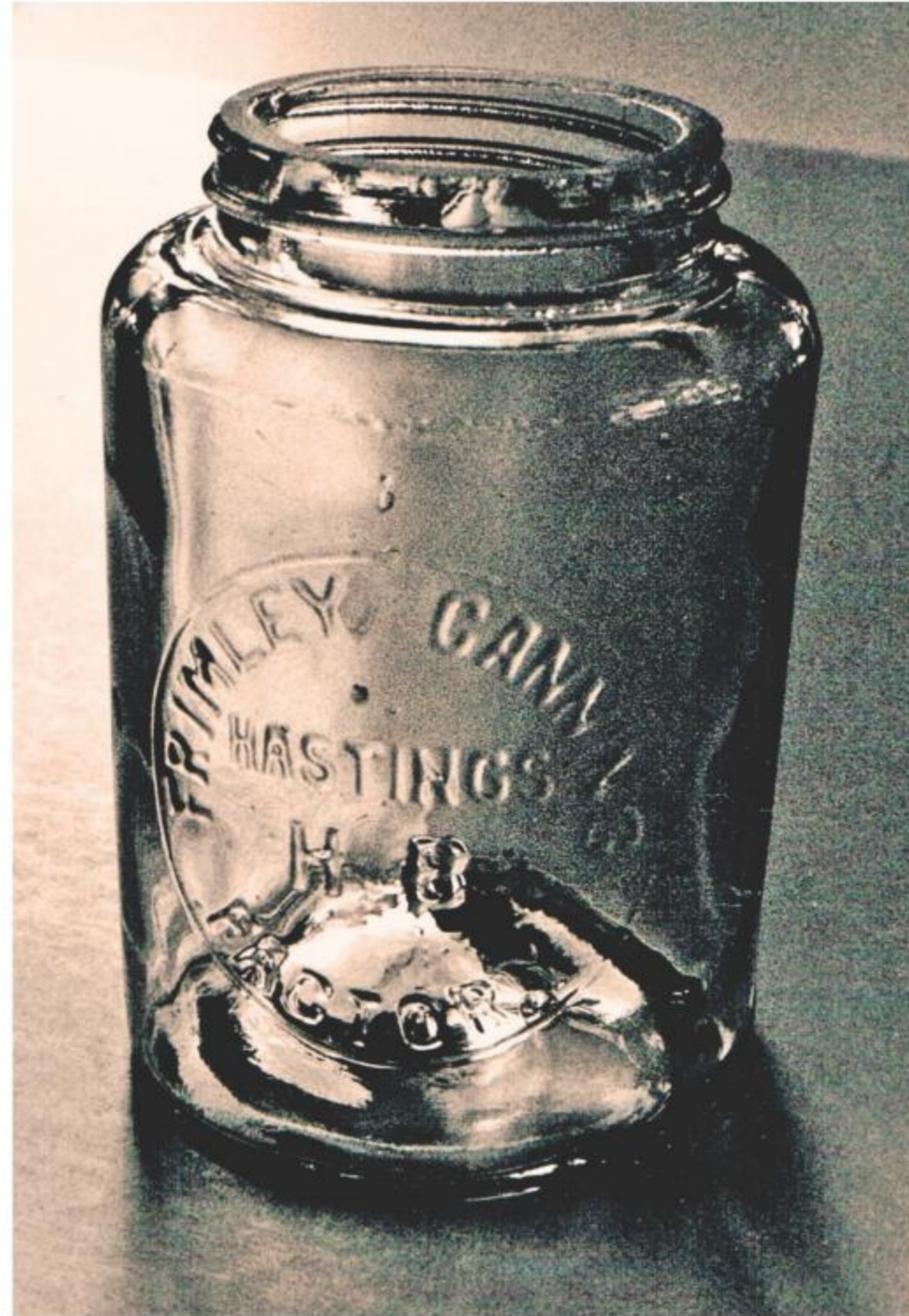
2lb clear glass, squarer shoulders 135mm x 92mm. Neck & body seams match. Definite mould seam on shoulder. 4 piece mould.
