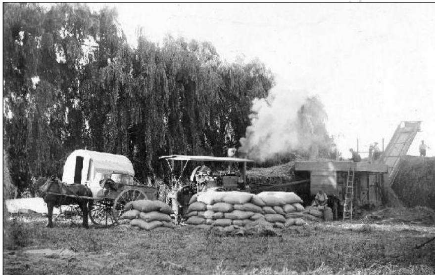
1900, Powdrell Brother's, carriers and expressman firm at Hastings, their new traction engine operating a thrashing machine at Hastings
