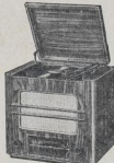
The 321 is a 5-tube All-Wave Superheterodyne set. Superior tone quality was put first and foremost when Philips designed this new All-Wave radioplayers. To achieve this for both fidelity and selectivity, there were several conditions that had to be met. The result is a radio that gives world-wide coverage — a reproduction of the original performance.
