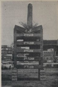
BOMB DOOR TESTS.—A 100 lb. bomb being placed only five floors during the experiment in London to test the value of bomb defectors.
