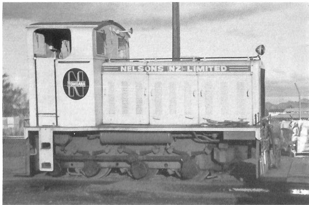
BELOW: Ex-NZR "Tr" class diesel shunting tractor No. 23 (Drewry 2126 of 1939) was purchased by Nelsons in 1981 and was photographed at Tomoana on 1 June 1983. (Photograph: P. F. Dyer)
