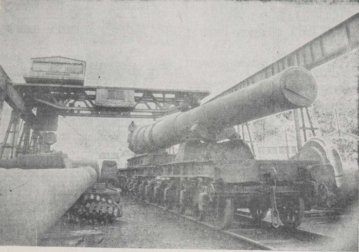
ON THE WAY.—People would be surprised to know how few shots a 16-inch gun-barrel can fire before it wears out. Hence the necessity for constant renewals. Here is one on its way to fill a gap in the turrets of a British warship.
