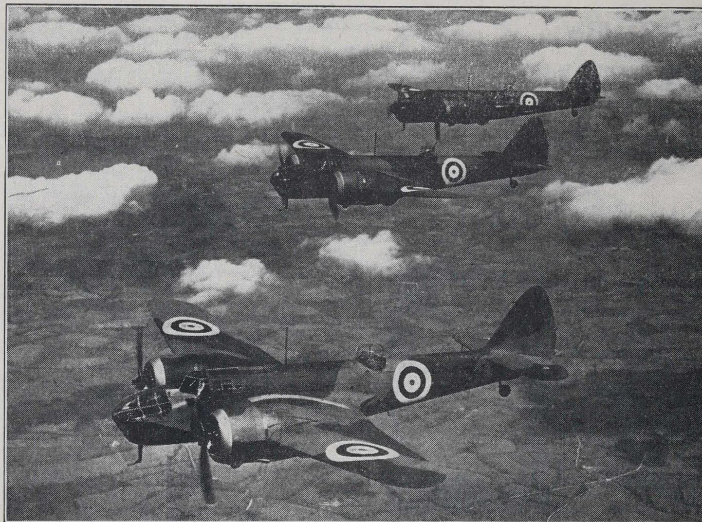
THE SPEARHEAD OF THE R.A.F. ATTACK. —These Bristol Blenheim medium bombers represent a magnificent achievement in aircraft design and are the pride of the R.A.F. They can carry their load of bombs nearly 2000 miles non-stop, and have a top speed of 300 miles an hour. Fast, and with great manoeuvrability, they are more than a match for many of the enemy fighters.
