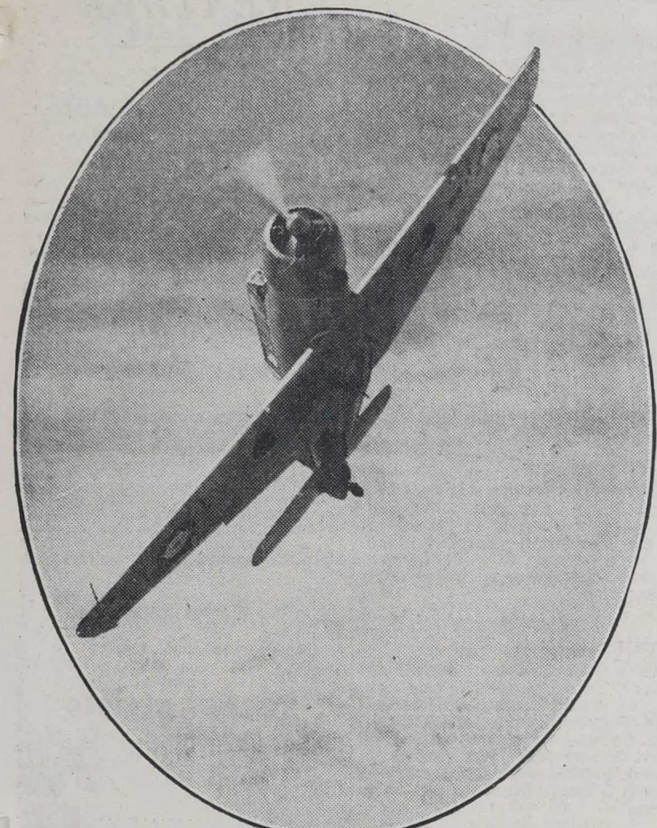
DIVE BOMBER. —A Blackburn Skua dive bomber pulling out of a dive. It carries its bombs slung under the fuselage, launching them at the end of a steep dive on the target. These formidable attack machines are also used extensively by the Fleet Air Arm, which controls all aircraft carried on ships.
