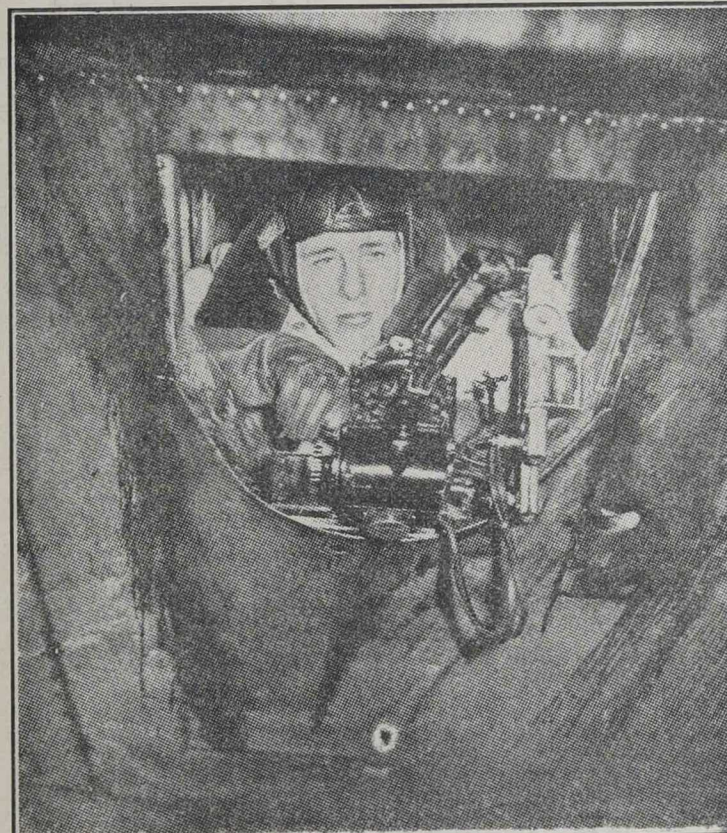
THE BOMB AIMER. —In some of the light bombers the bomb aimer lies on the floor to operate his bomb sight. Calculations of height, speed, windage, etc., are recorded on the bomb sight, and the moment at which to release the bombs is thus determined.
