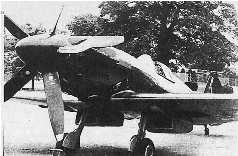
A Spitfire PR.19 showing its five-bladed propeller and the Griffon engine installation
